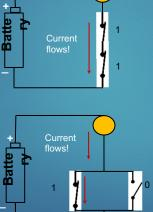
Both switches must be "on" for current to flow from + to -(for bulb to light up) (AND)
