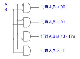
2-bit decoder (4 input decoder)
